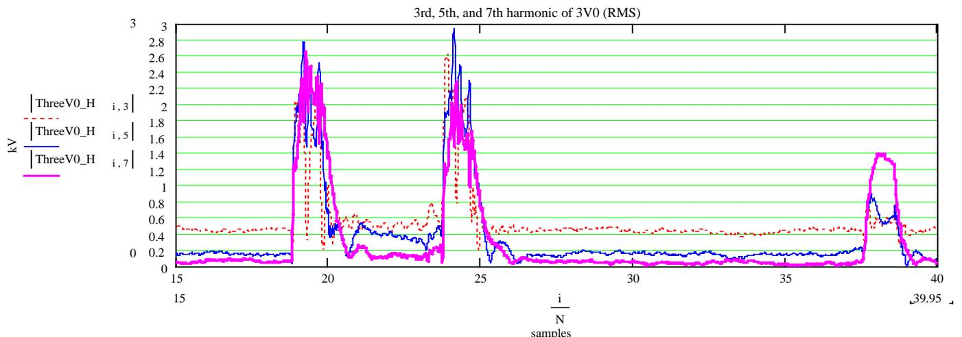
Figure 6. 3<sup>rd</sup>, 5<sup>th</sup>, and 7<sup>th</sup> harmonics of the 3V0 voltage (RMS).
