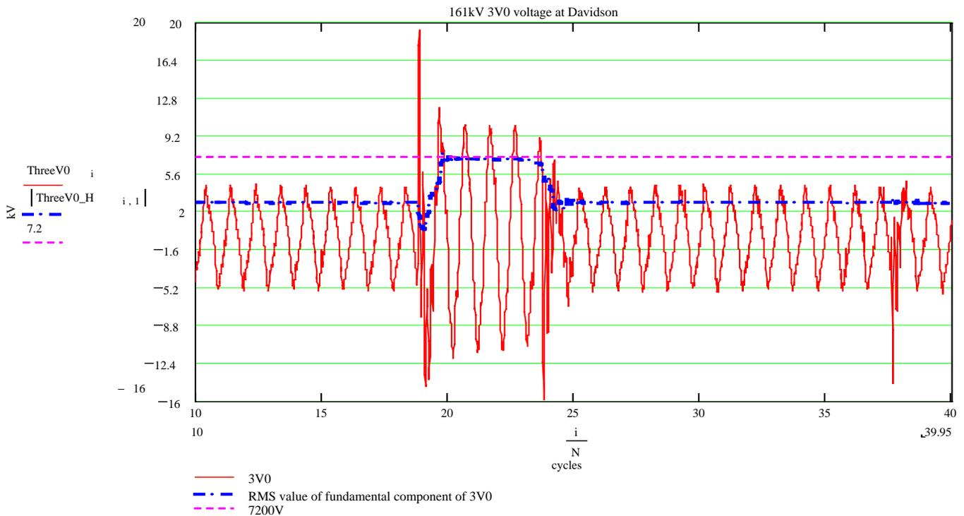
Figure 4. Graph of 161kV 3V0, RMS of fundamental component, and SV pickup.
