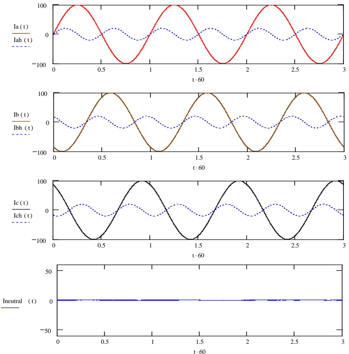
Below are 3 cycle plots of A, B, and C 60Hz phase currents along with a 20% 3<sup>rd</sup> harmonic that might be superimposed on these waveforms. The 3<sup>rd</sup> harmonic is a zero sequence (triplen) harmonic so the components in each of the three phases sum to three times in the neutral.
