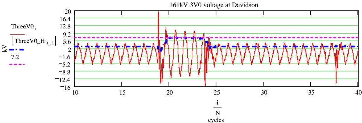
Note: Importing ASCII COMTRADE data is as easy as reading comma separated data. There are several methods of reading data into Mathcad. The path chosen in this data file (see VA:= input equation at top) references the first column of data as column 0. The A-phase voltage is at column 3 so it is referenced as 2. The data is scaled as per C37.111 by the "a" constant of "0.145064" from the associated CFG file. This satisfies the equation ax+b with b = 0 in the CFG file.
